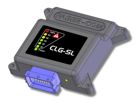
Overall dimensions: 138 x 110 (147 with connector) x 38 mm
